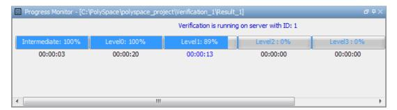
The progress monitor highlights the current phase in blue and displays the amount of time and completion percentage for that phase.
